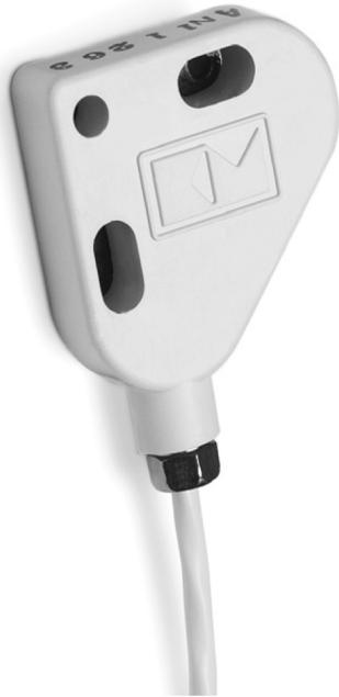
The L-Cell is a bolt-on strain gage sensor that is uniquely designed, highly sensitive, thermally stable, dual axis strain gage sensor which is bolted directly to the vessel's support structure. The L-Cell® measures changes in stress in the vessel support member and provides a change in voltage output in direct proportion to the weight of material.
